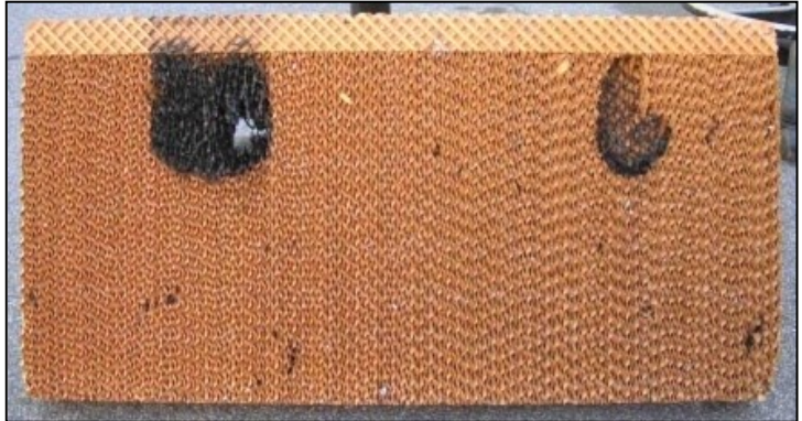
Figure 2. A roof mounted evaporative air conditioning unit. Figure 3. A cellulose filter pad exposed to ember attack (during testing)
