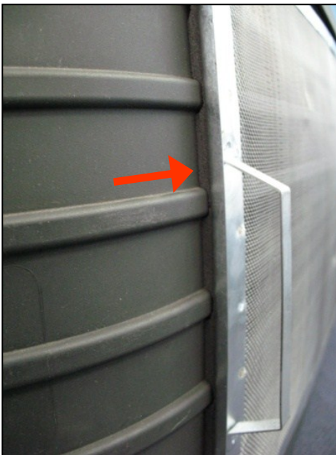
Figure 6. A sealant is used to fill any gaps
