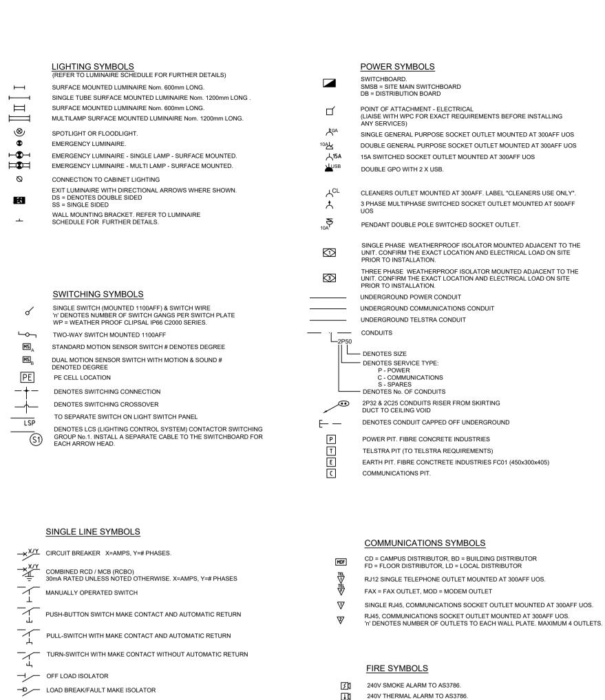
A/B HRC FUSE A = CARTRIDGE SIZE, B = HOLDER RATING
