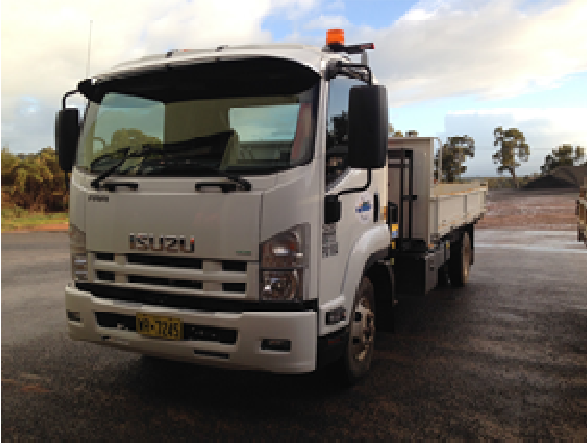
The new Isuzu works truck replaces the very old seven tonne truck and offers much greater flexibility, being equipped with a crane, three way tipper (end tips as well as to either side), and various storage compartments and racks
